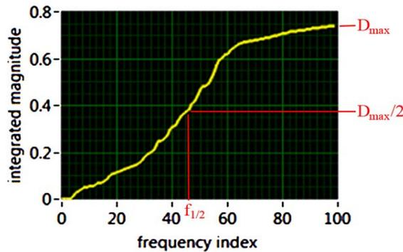
Figure 6. Cumulative distribution function showing extraction of  $D_{max}$  and  $f_{1/2}$ .
