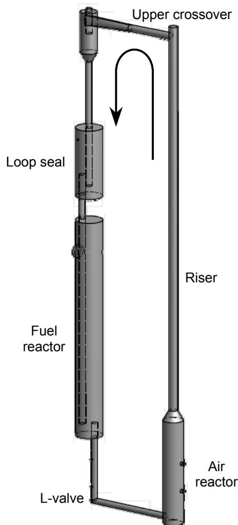
Figure 1. Chemical looping reactor at NETL. The Doppler sensor is located in the upper crossover. The arrow shows the direction of particle circulation. The thermal insulation and outer housing is not shown.
