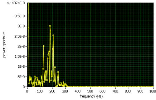
Figure 5. Frequency spectrum from 150  $\mu\text{m}$  diameter ilmenite particles falling 2.1 m, horn angle 52 degrees; 10 GHz source.
