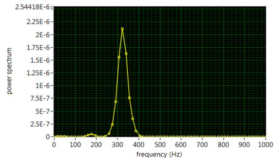
Figure 4. Frequency spectrum from a steel ball 0.157" diameter falling 1.8 m, horn angle 42 degrees; 10 GHz source.
