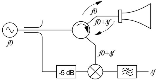
Figure 2. Block diagram of the microwave electronics.
