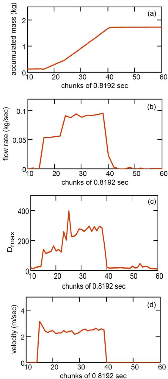
Figure 7. Data from room-temperature measurements of an ilmenite particle flow: (a) accumulated mass as a function of time; (b) mass flow rate measured using the accumulated mass; (c) extracted  $D_{max}$ , a measure of the particle density; and (d) particle velocity extracted from the measurements.
