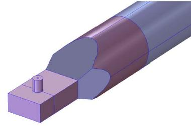
Figure 3. Microwave launcher showing transition from coaxial cable to circular waveguide.
