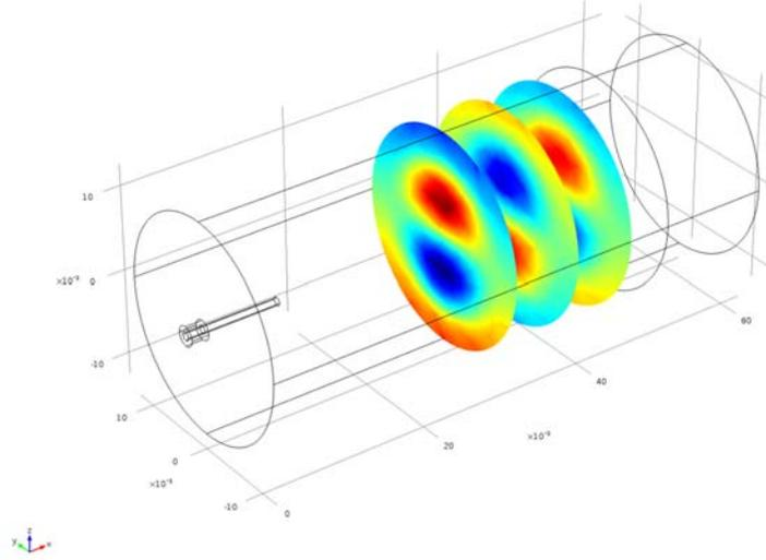
Figure 5. Excitation of a circular waveguide with a small end probe. The color indicates the  $H_y$  component.
