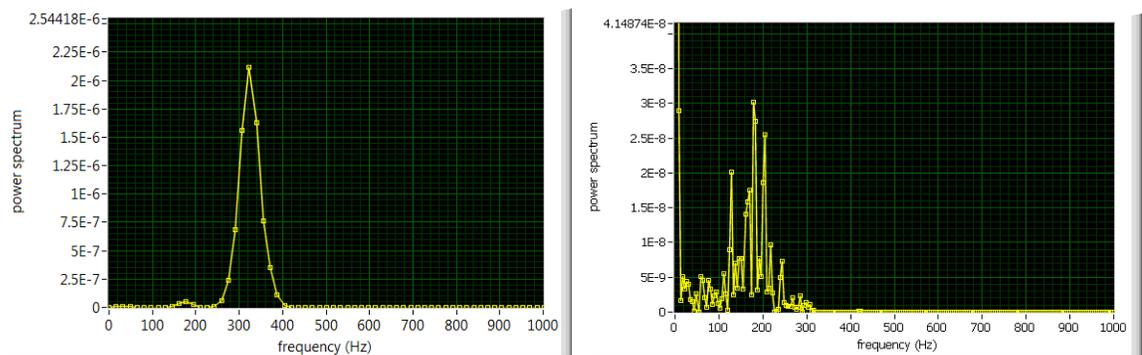
Figure 4. Fourier power spectrum calculated from mixer output signal: (left) 0.157" diameter steel ball, and (right) ilmenite from table feeder.
