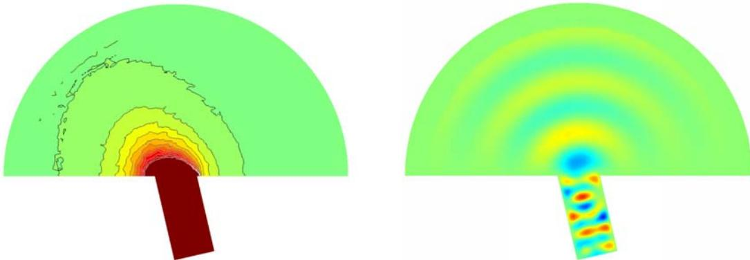
Figure 8. Results of simulation of microwave launch from alumina cylinder into air: (left) contours of constant time-averaged energy density and (right) electric field normal to the surface.
