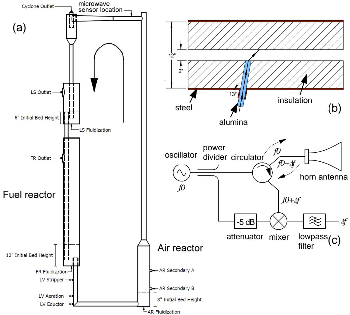
Figure 2. The Doppler flow sensor: (a) outline drawing of the NETL cold flow reactor showing the sensor location; (b) detail drawing showing the insulation around the flow region and the microwave launcher; and (c) block diagram of the microwave circuit.
