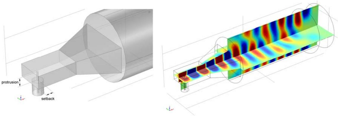
Figure 6. Geometry of the tapered coaxial to circular waveguide transition (left) and simulated  $x$  component of the electric field (right).
