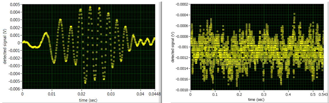
Figure 3. Mixer output signal as a function of time: (left) steel ball 0.157" diameter falling 1.8 m, horn angle 42°; (right) ilmenite from table feeder falling 2.1 m, angle 52°.
