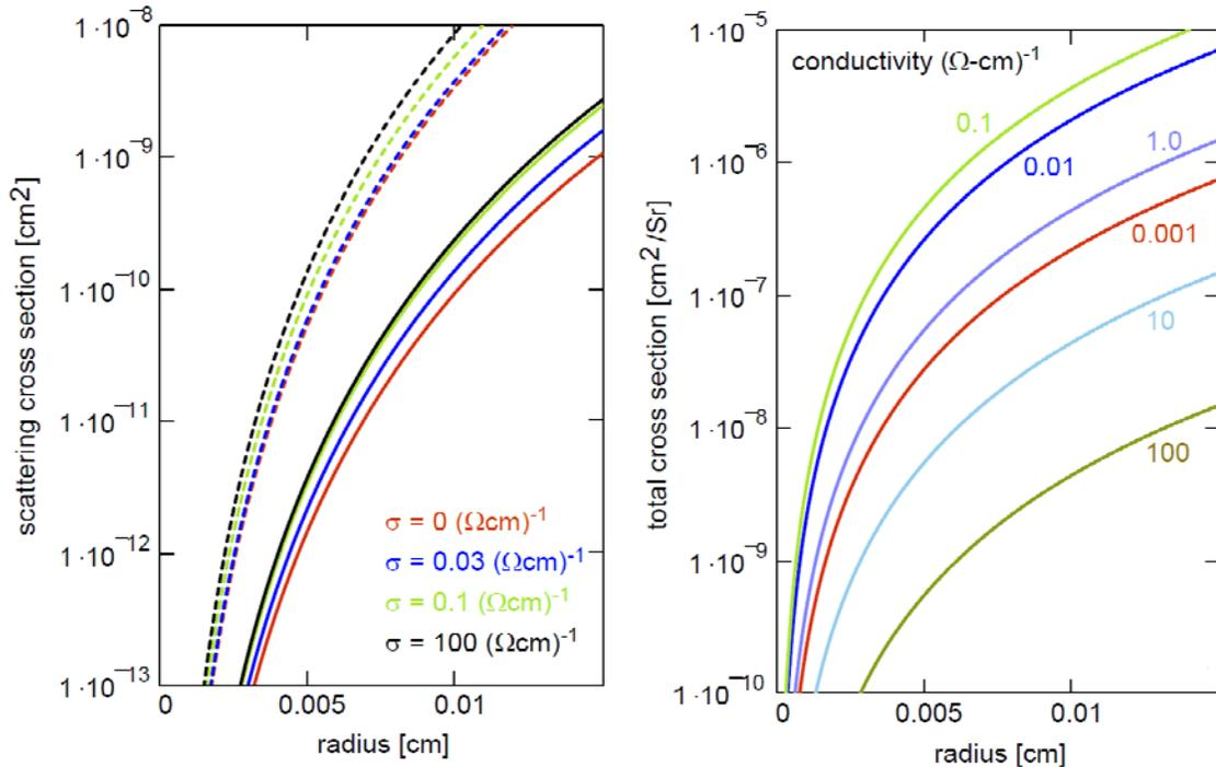
Figure 1. Predictions from the Rayleigh theory for scattering from spherical ilmenite particles. (Left) total scattering cross section as a function of particle size and electrical conductivity. Solid lines are for 10 GHz and dashed lines 24 GHz. (Right) absorption cross section at 10 GHz. The absorption cross section has a non-monotonic dependence on electrical conductivity.
