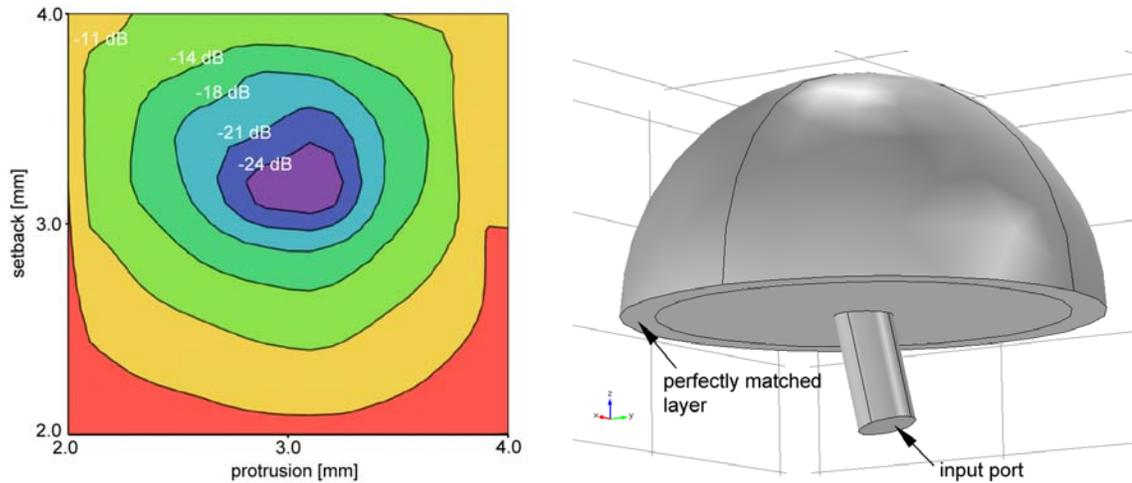
Figure 7. (Left)  $S_{11}$  as a function of probe protrusion and spacing from the back wall for the tapered coaxial to waveguide transition; and (right) geometry for simulating launch of microwaves into air from an alumina cylinder.
